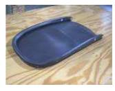
Cutting Dynamics, Inc. (CDI), has developed the most cost-effective means for processing lightweight thermoplastic advanced composite components for seatbacks used by the aerospace industry. CDI uses a unique high-speed moulding process to produce a complex-geometry hollow structure for seatbacks from braided thermoplastic slit tape.
